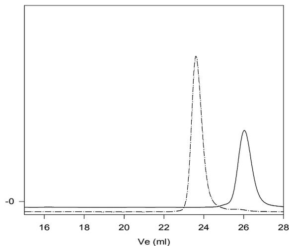
Size exclusion chromatography of polystyrene-b-polyisoprene, 1,4 addition
