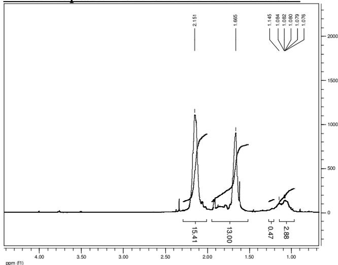
**<sup>1</sup>H-NMR Spectrum of the block copolymer:**
