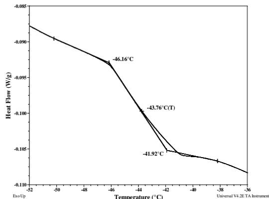
**Melting and crystallization curve for the sample**
