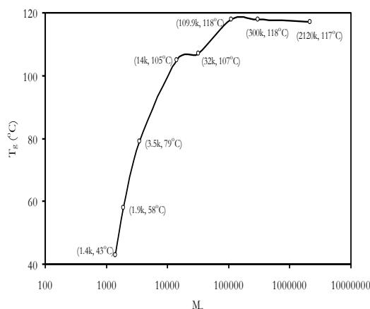
**T<sub>g</sub> vs MW for selected poly t-butyl methacrylate**
