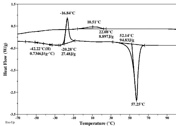
**DSC thermograms of the polymer (3<sup>rd</sup> heating scan, 10°C/min):**
