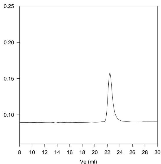
Size exclusion chromatograph of polymethylmethacrylate-rich in atactic: M<sub>n</sub>=42,000, M<sub>w</sub>=47,000, PI=1.12
