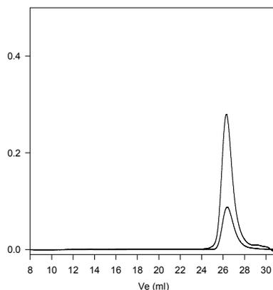
Size exclusion chromatography of poly(butadiene-b-ethylene oxide):
