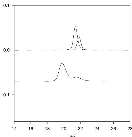
**Size Exclusion Chromatography :**—— First PS block,  $M_n=65,000$ ,  $M_w/M_n=1.05$ —— PS2Vp, the diblock PS(65,000)-b-P2Vp(60,000),  $M_w/M_n=1.06$ —— PS2VpEO, the triblock PS(65,000)-b-P2Vp(60,000)-b-PEO(105,000)  $M_w/M_n=1.14$
