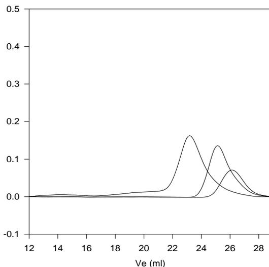
Size exclusion chromatography of ω-α dihydroxy in the center polystyrene and after reaction with Caprolacton
