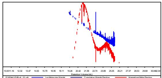
After Hydrolysis of Ester - PS-b-AA: Mn 26,000-b-76,000 Mw/Mn 1.2
