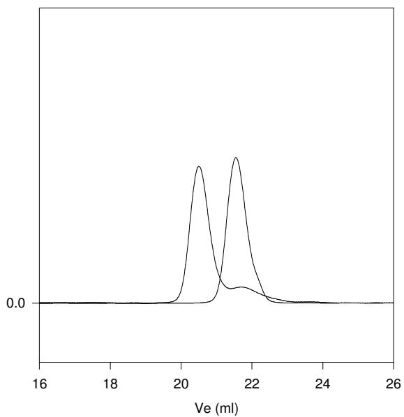
Size exclusion chromatography of poly(butadiene-b-ethylene oxide):
