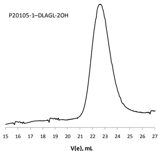
SEC elution of the dicarboxy functionalized polymer is retarded in our set of columns. This may be due to strong interaction of the carboxyl functional groups of polymer chains with the column packing material.
