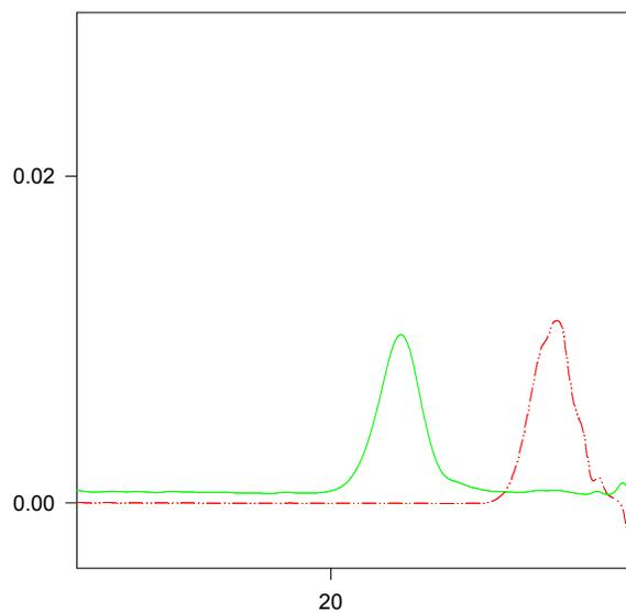
Size exclusion chromatography of poly(2-Hydroxy ethylacrylate(protected with TMS)-b-neopentylmethacrylate)
