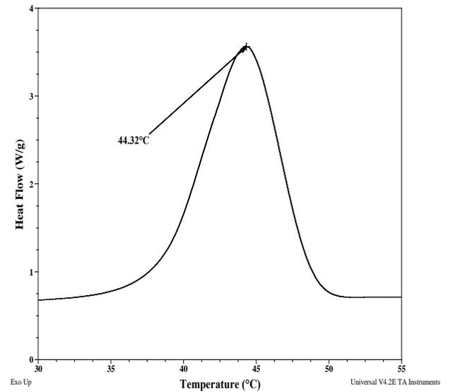
**Melting and crystallization curve for the PEO block**
