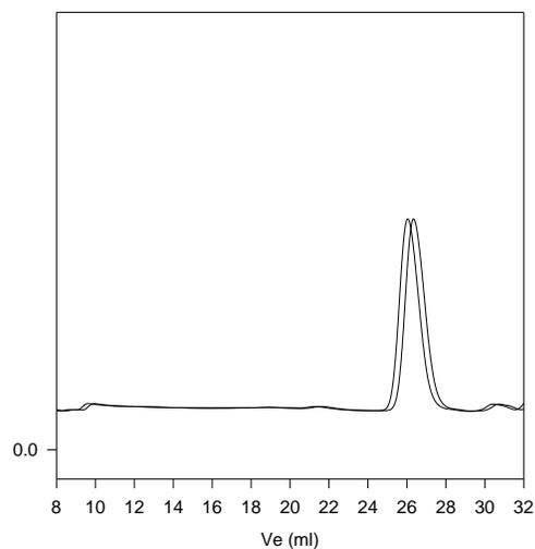
Size exclusion chromatography of poly(butadiene-b-ethylene oxide):
