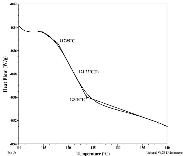
**T<sub>g</sub> of homopolymer MMA as function of M<sub>n</sub>**
