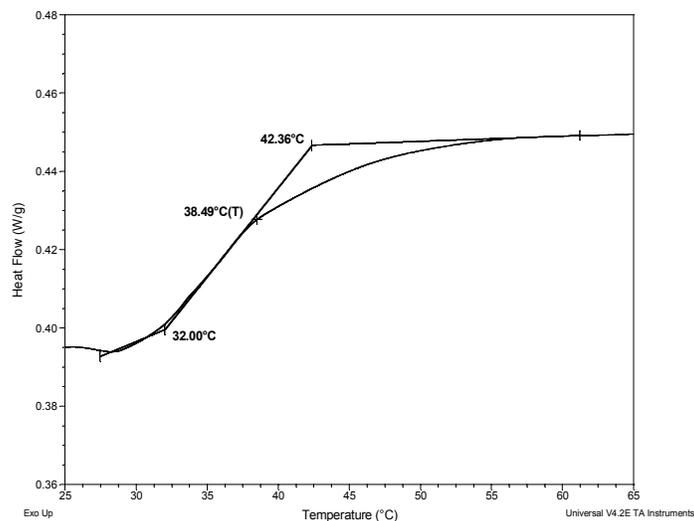
**Thermogram for PMMA block polymer**
