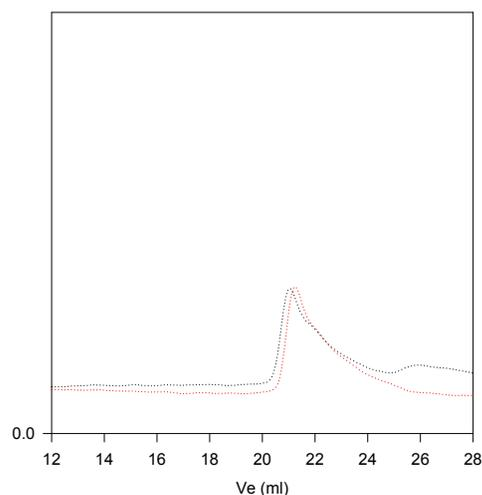
Size exclusion chromatography of poly(methyl methacrylate-b-N,N-dimethyl acrylamide) in DMF at 40 °C containing 0.01M LiBr as additive
