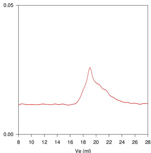
Size exclusion chromatography of  $\omega$ - $\alpha$  dihydroxy Terminated polystyrene:
