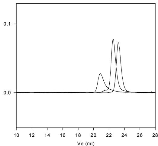
Size exclusion chromatography of polystyrene-*b*-butadiene (rich 1,2 addition)-*b*-methylmethacrylate)
