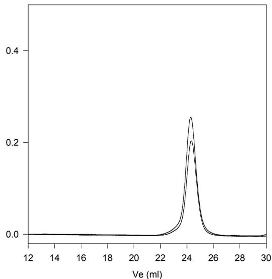
Size exclusion chromatography of polystyrene-b-polyisoprene<sub>1,4 addition</sub>
