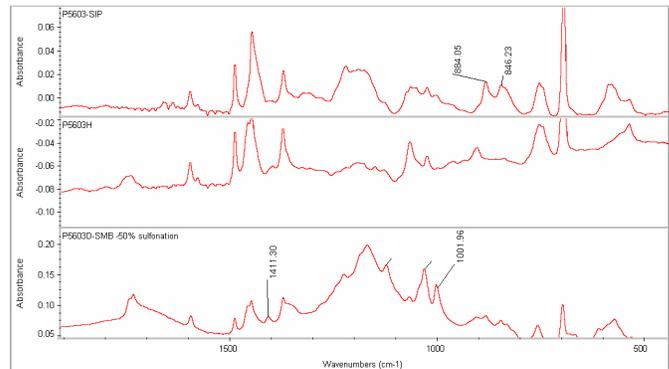
In Hydrogenation: The characteristics at 885 and 846cm<sup>-1</sup> should be disappeared.
