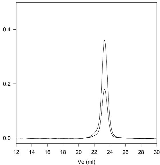
Size exclusion chromatography of polystyrene-b-polyisoprene<sub>1,4</sub> addition
