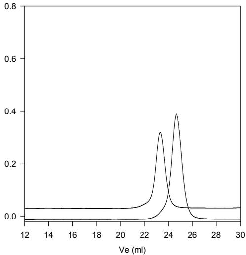
Size exclusion chromatography of polystyrene-b-polyisoprene<sub>1,4</sub> addition
