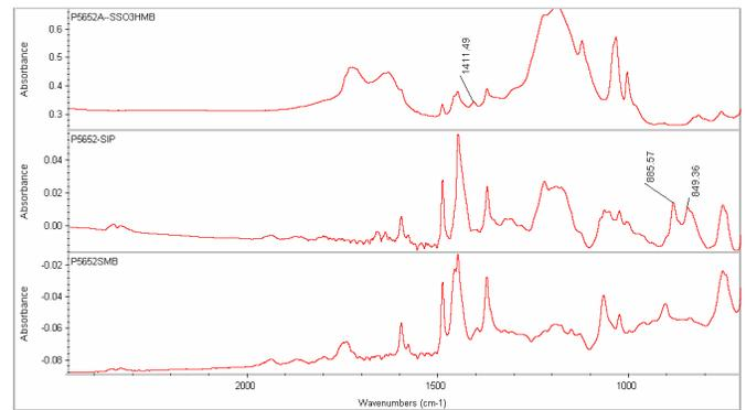
In Hydrogenation: The characteristics at 885 and 846 $cm^{-1}$  should be disappeared.
