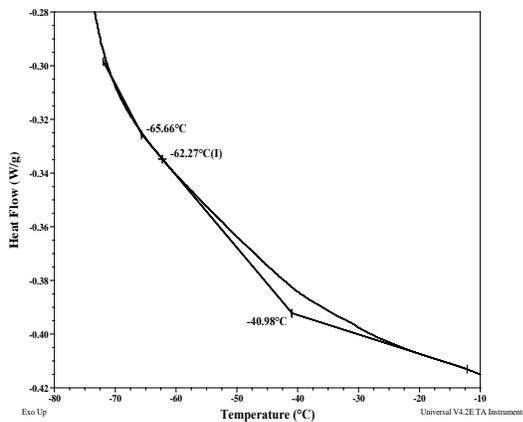
**Melting and crystallization curve for the PEO block**
