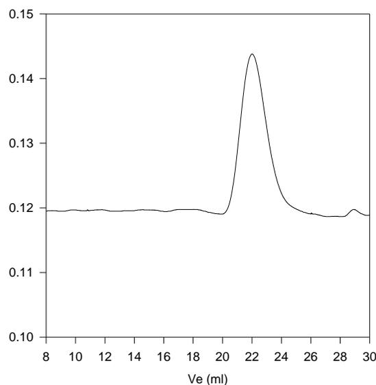
Size exclusion chromatograph of polymethylmethacrylate-rich in atactic: M<sub>n</sub>=30,000, M<sub>w</sub>=42,000, PI=1.4
