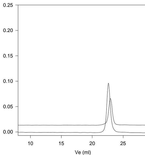
Size exclusion chromatography of poly(styrene-b-ethylene oxide contain C13 label ethylene oxide:15%)
