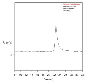
Size Exclusion Chromatography of Poly isoprene deuterated  $M_n = 41,000, M_v = 49,000, M_v/M_n = 1.2$  data from light scattering detector:
