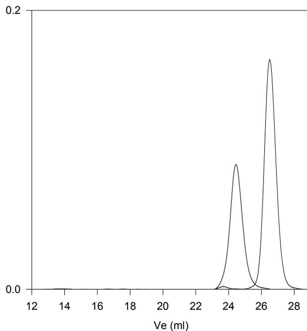
— Poly(ethylene oxide),  $M_n=2000$ ,  $M_w=2100$ ,  $PI=1.05$
