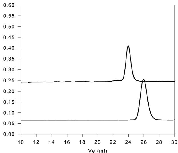
— Poly(methyl methacrylate): M<sub>n</sub>=3000, M<sub>w</sub>=3500, M<sub>w</sub>/M<sub>n</sub>=1.2
