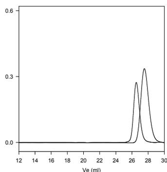
Size Exclusion Chromatogram of Poly(butadiene-b-ethylene oxide)
