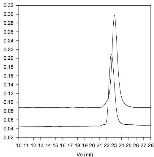
— Polystyrene, M<sub>n</sub>=26000, M<sub>w</sub>=30,500, PI=1.18
