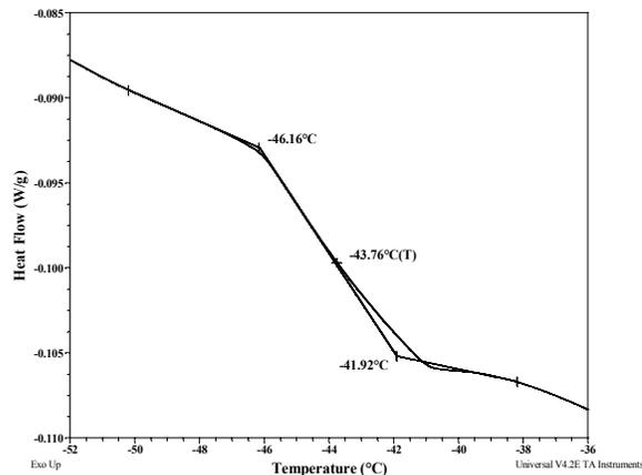
**Melting and crystallization curve for the sample**
