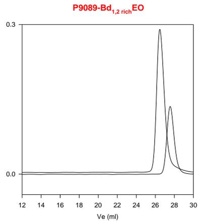
Size Exclusion Chromatogram of Poly(butadiene-*b*-ethylene oxide)
