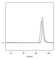
Polystyrene, M.=22,000, M.=23,000. PI=1.05 Block Copolymer PS(22,000)-b-P4VP(21,600), PI=1.15 Composition from H NMR
