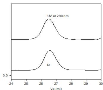
Size exclusion chromatography of poly(ethylene glycol) methyl ether styrene with ultraviolet (UV) and refractive index (RI) detectors
