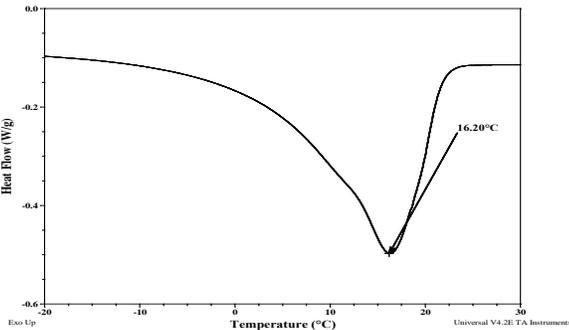
**Crystallization curve for the sample:**
