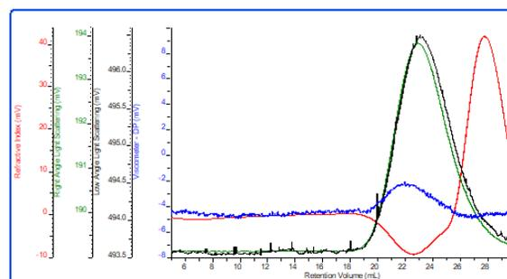
GPC run in DMF Shows first RI negative response and the values are overestimated. The Mw/MN values were calculated by SEC and Mn value determined by HNMR analysis.
