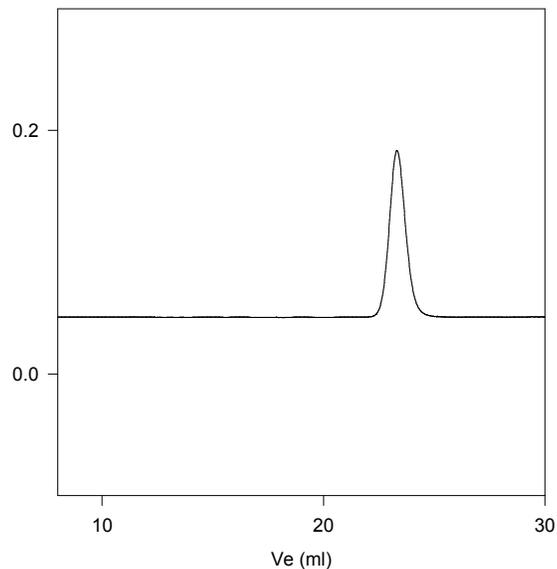
— Polystyrene, M<sub>n</sub>=23,000, M<sub>w</sub>=24,500, PI=1.07
