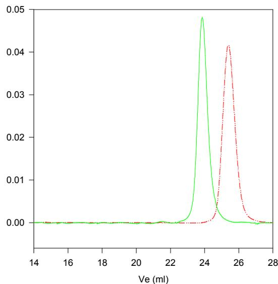
Size exclusion chromatography of poly(Popylene oxide-b-Ethylene Oxide):
