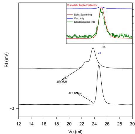
Size Exclusion Chromatography of four arm poly(ethylene oxide)
