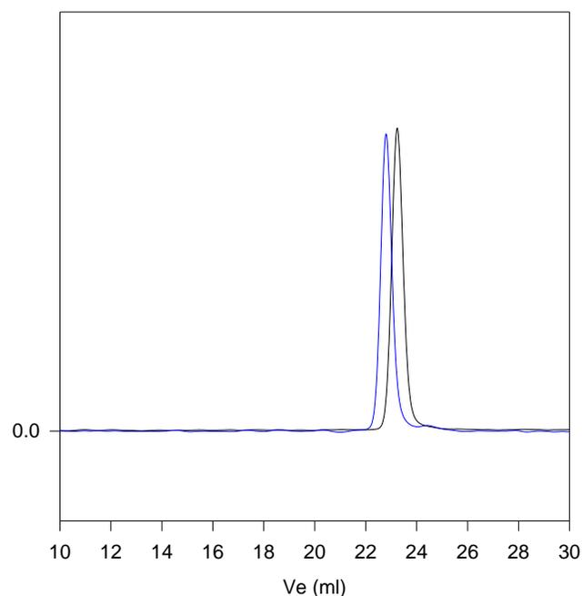
Size exclusion chromatography of poly(isoprene-b-ethylene oxide)
