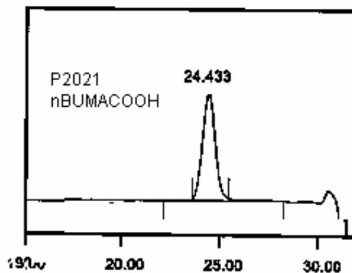
Size exclusion chromatography of poly(n-butyl methacrylate) (before terminating reaction with  $\text{CO}_2$ )
