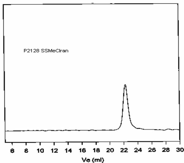
Size exclusion chromatograph of random copolymer of Poly(styrene-co-p chloromethylstyrene):
