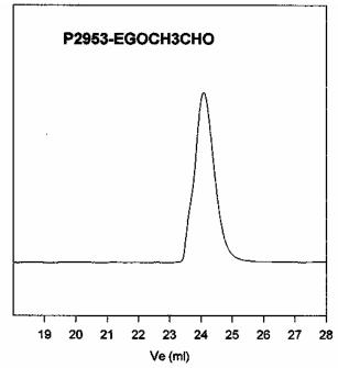
Size exclusion chromatography of functionalized α-formyl-ω-Methoxy terminated Poly(ethylene glycol):
