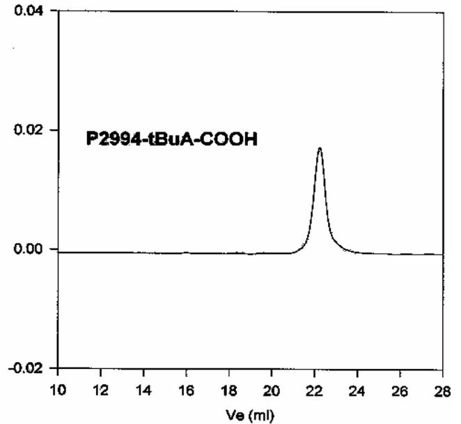
Size exclusion chromatography of poly(tert.butylacrylate) (before terminating reaction with CO<sub>2</sub>).
