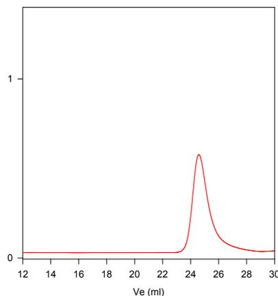
Size exclusion chromatograph of copolymer of Poly(styrene-co-4-hydroxy styrene)random copolymer
