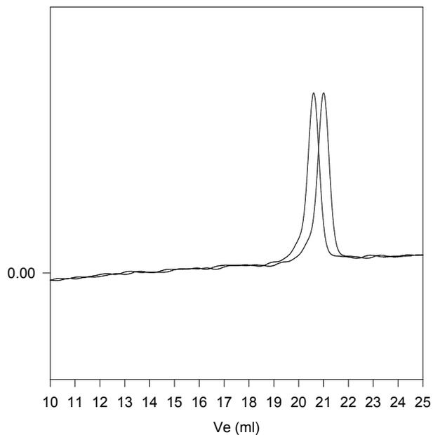
Size exclusion chromatography of poly(styrene-b-ethylene oxide)
