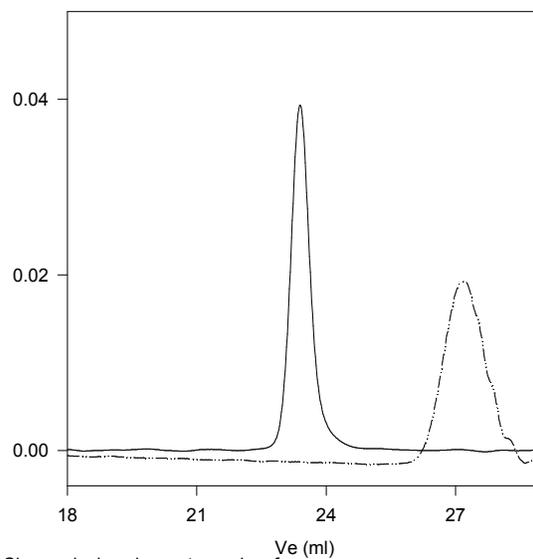
Size exclusion chromatography of poly(2-Hydroxy ethylmethacrylate(protected with TMS)-b-neopentylmethacrylate)
