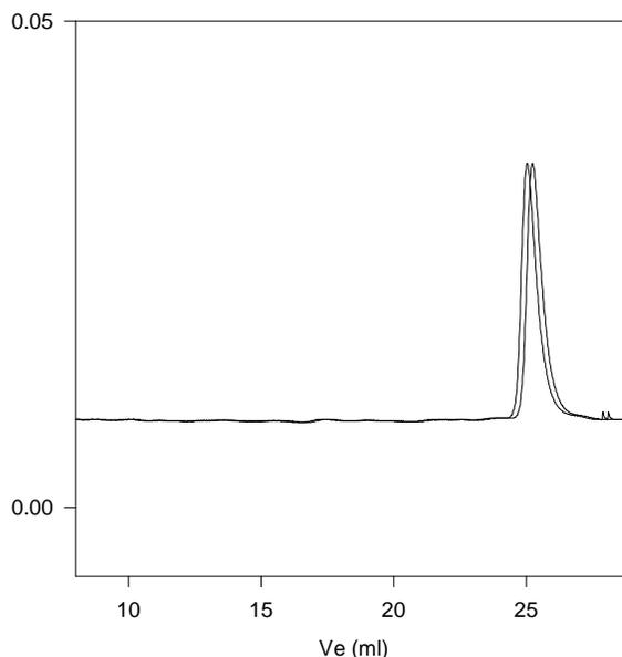
Size exclusion chromatography of poly(styrene-b-ethylene oxide)
