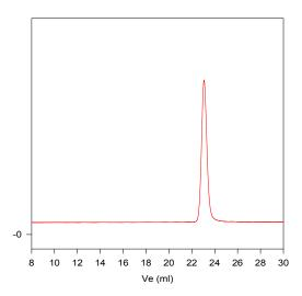
Size exclusion chromatograph of poly(styrene sulfonic acid-Sodium salt)
