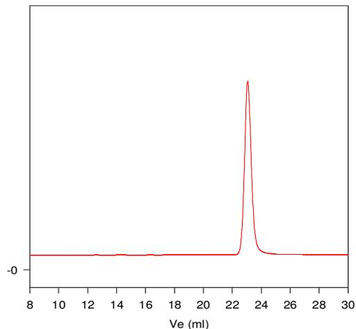
Size exclusion chromatograph of poly(styrene sulfonic acid-Sodium salt) Polystyrene precursor
