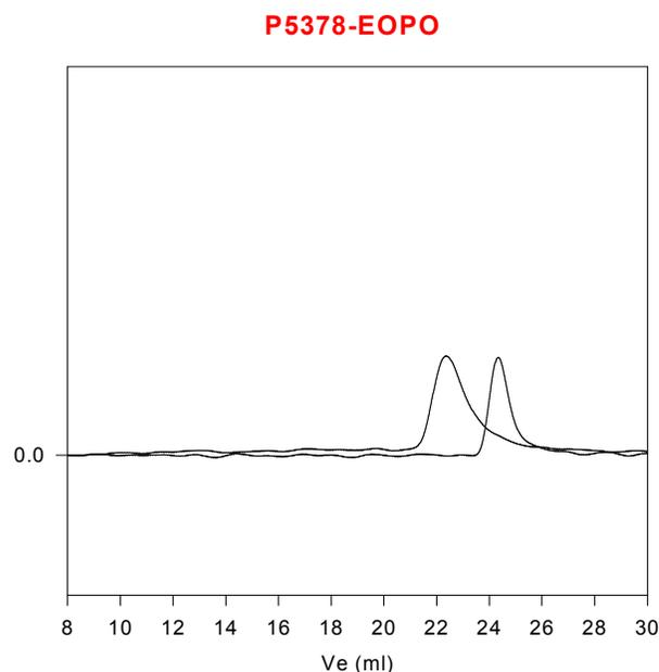
Size exclusion chromatography of poly(Popylene oxide-b-Ethylene Oxide):
